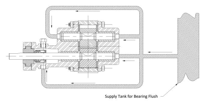
A bearing flush can be used to provide better lubrication and heat dissipation at lower viscosities, or to allow the bearings and containment can to flood more quickly at higher viscosities.
