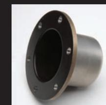
**CONTAINMENT CAN** The standard containment can is made of Alloy-C, a high nickel alloy which is 40% stronger than Stainless Steel. Alloy-C has the added benefit of minimizing magnetically induced eddy current power losses that can add heat to the pumped product. The Poly-Guard™ is also offered
